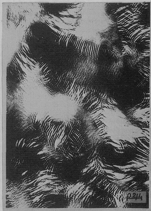
Figure 8. Electron micrograph of an unannealed film of the (SB) 6 -DVB-1 star block copolymer. Film cast from a 9/1 tetrahydrofuran-methyl ethyl ketone mixture. The large white areas are the result of delamination during microtoming.
